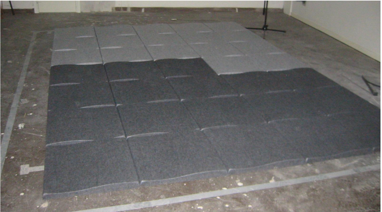
Wall panels mounted on the floor of the reverberation room.
